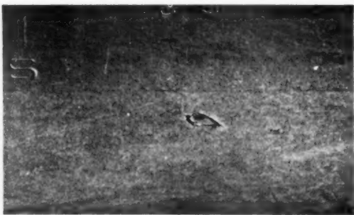
Fig. 10—Acid-etched defect, previously almost invisible, which leaked at only 3,000-psi. testing pressure.
